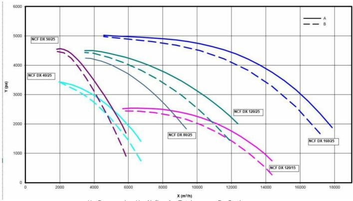
Y = Pressure drop X = Air flow A = Total pressure B = Static pressure
